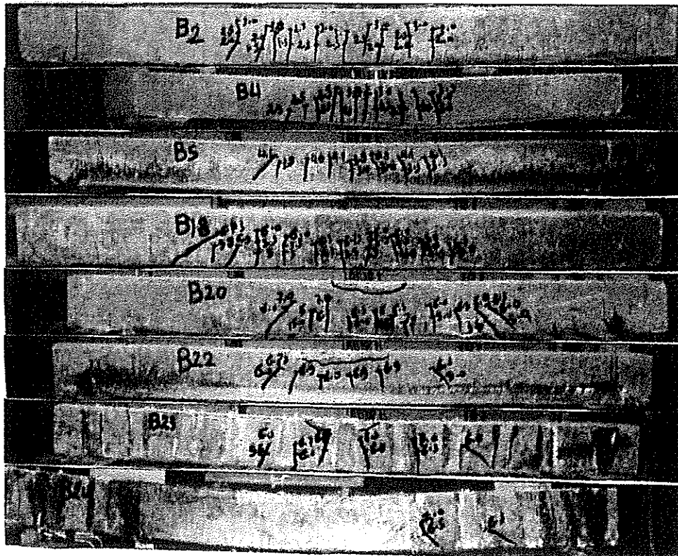
Fig.(10) The crack pattern of some of the tested beams at failure
