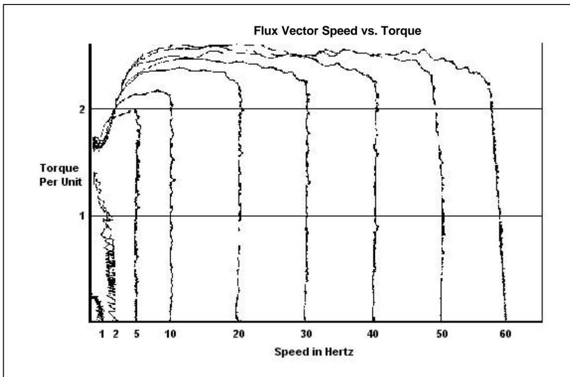
This graph shows the steady state torque capability of a flux vector drive. The speed control has been improved. Second, the torque output capability is better. Note however that there is still a decrease in the available torque at low speeds. This occurs primarily because the drive still contains the volts/hertz core.
