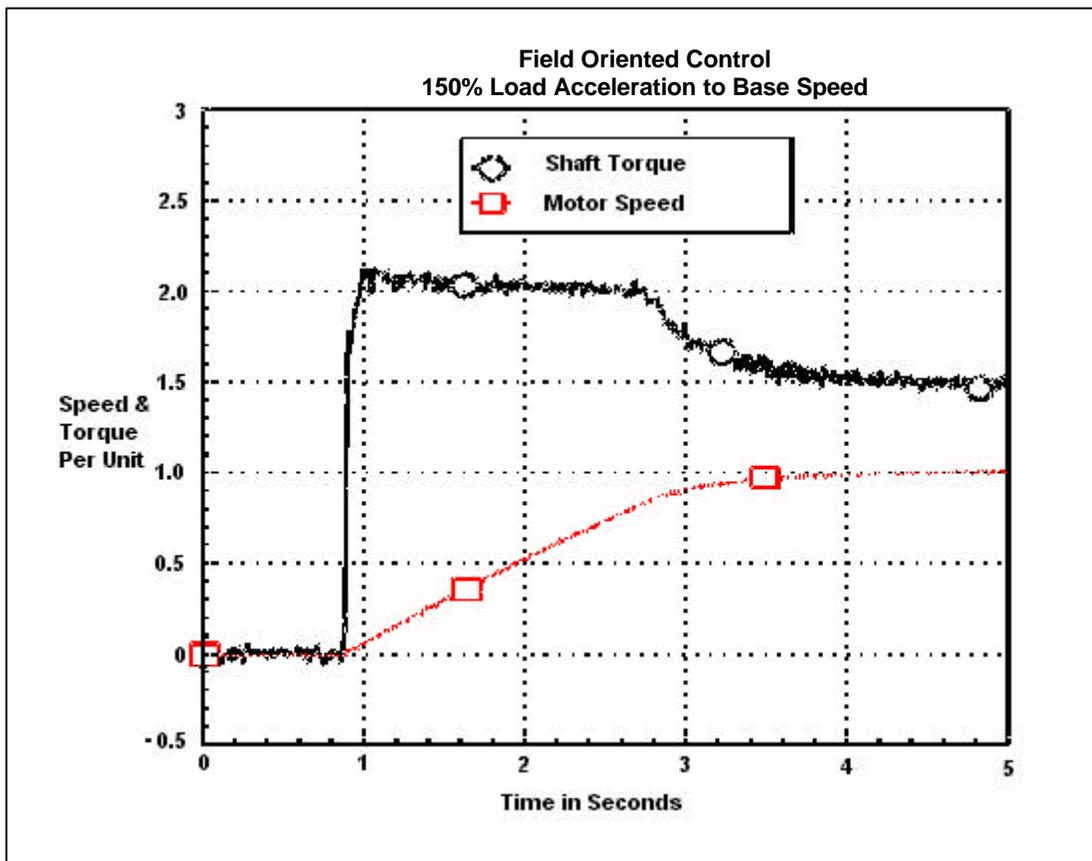
This graph shows the ability of a drive using Force Technology to maintain control over torque and speed, even under extreme conditions.
