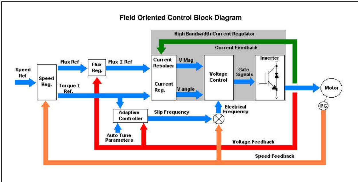
A high bandwidth current regulator that separates and controls the components of stator current replaces the volts/hertz core. The high bandwidth characteristics of this control help eliminate nuisance trips due to shock-loads and will continuously adapt to changes in the motor and load characteristics.
