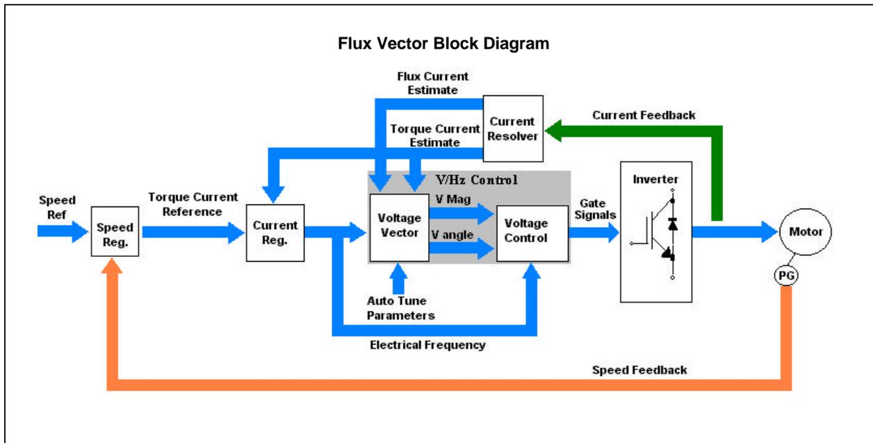
Recently, flux vector control has been enhanced to allow the drive to operate without the use of a speed feedback device, relying instead on estimated values for speed feedback and slip compensation. Again, the basic volts/hertz core is retained.
