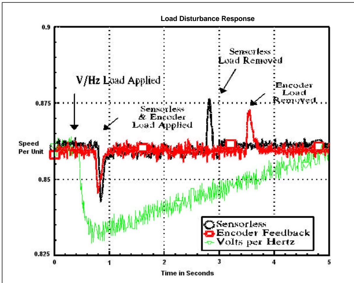
Contrast that against the volts/hertz response, which recovers much slower. The high bandwidth current regulators and high performance speed regulator ensure that the drive using Force Technology delivers high dynamic performance.
