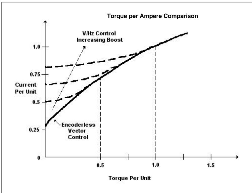
The result is that a motor run at low loads will dissipate higher losses when controlled by a volts/hertz drive. At slower speeds, this could cause unnecessary motor overheating.
