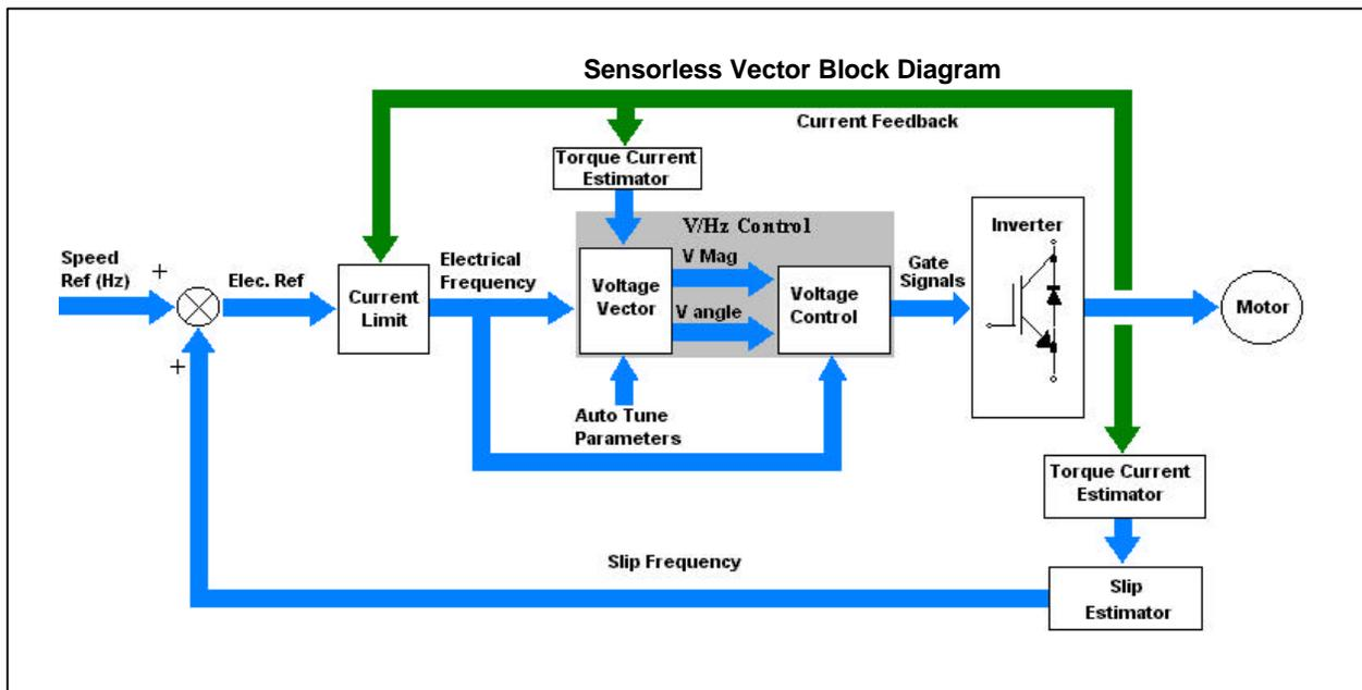
The control improves upon the basic volts/hertz control technique by providing both a magnitude and angle between the voltage and current. Volts/Hertz drives only control the voltage magnitude. Voltage angle controls the amount of motor current that goes into motor flux enabled by the Torque Current Estimator. By controlling this angle, low speed operation and torque control is improved over the standard volts/hertz drive.
