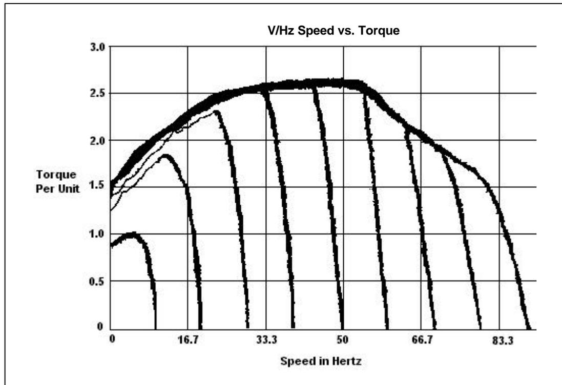
The plot above shows the steady state torque performance of a volts/hertz drive. A torque transducer directly on the motor shaft supplied the data that is plotted. The drive is given a fixed speed/frequency reference. Then load on the motor is increased and actual shaft torque is monitored.
